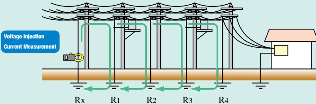
Clamp on the earth cable. The instrument has two cores for voltage injection and current measurement.
