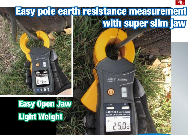
0.02  $\Omega$  to 1600  $\Omega$  wide measurement range for earth resistance measurement 1.00 mA to 60.0 A covering small leakage current to load current
